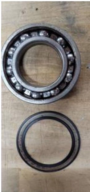
Figure 19: UUT5 Vented Bearing, Forced Humidity Post-Test Condition
