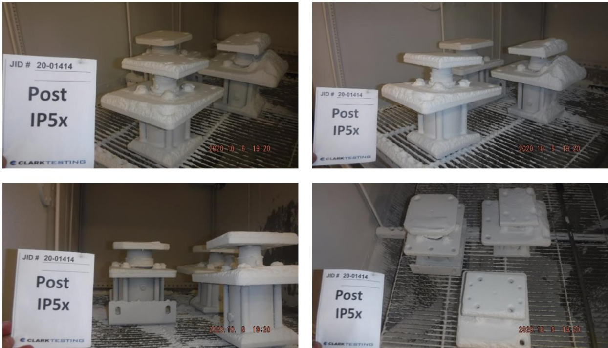
Figure 3: Dust Ingress Post-Test Condition
