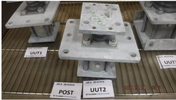
Figure 8: Humidity Post-Test Condition
