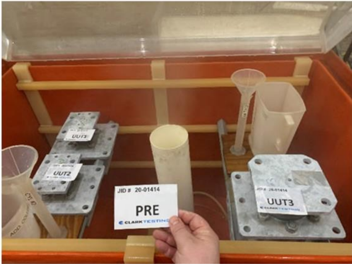
Figure 9: Salt Spray Pre-Test Condition
