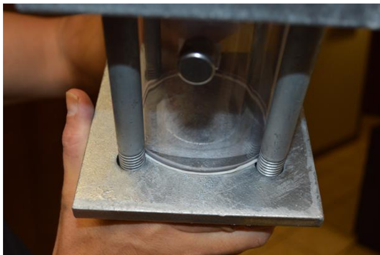
Figure 26: Field Test 4—Sealed, Vented Volume with One Teaspoon of Liquid Water
