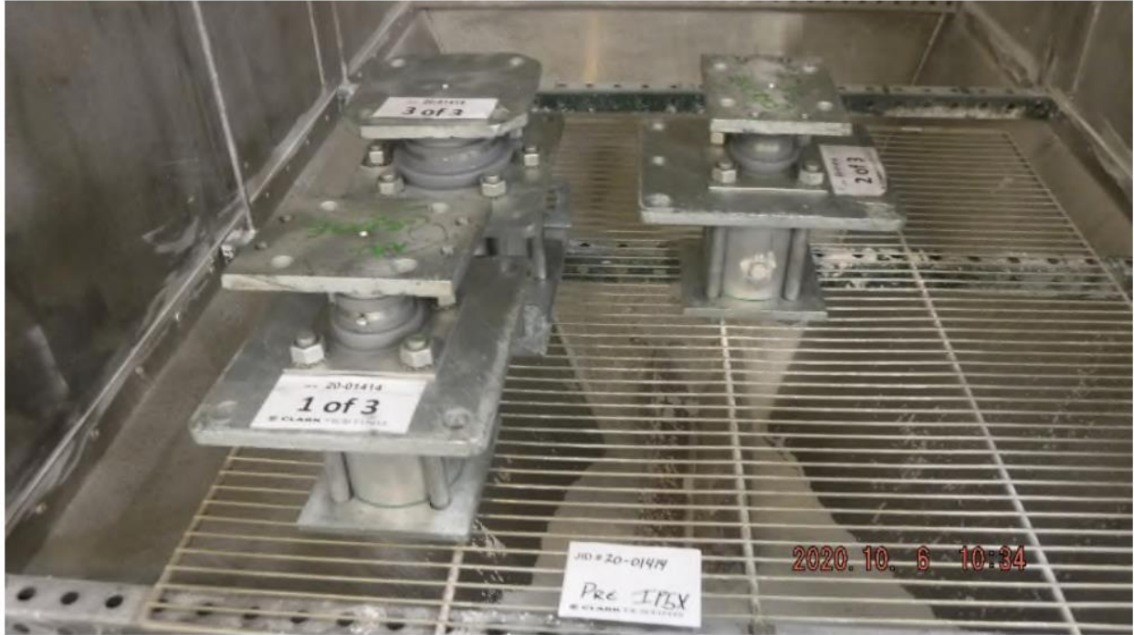
Figure 2: Dust Ingress Pre-Test Condition
