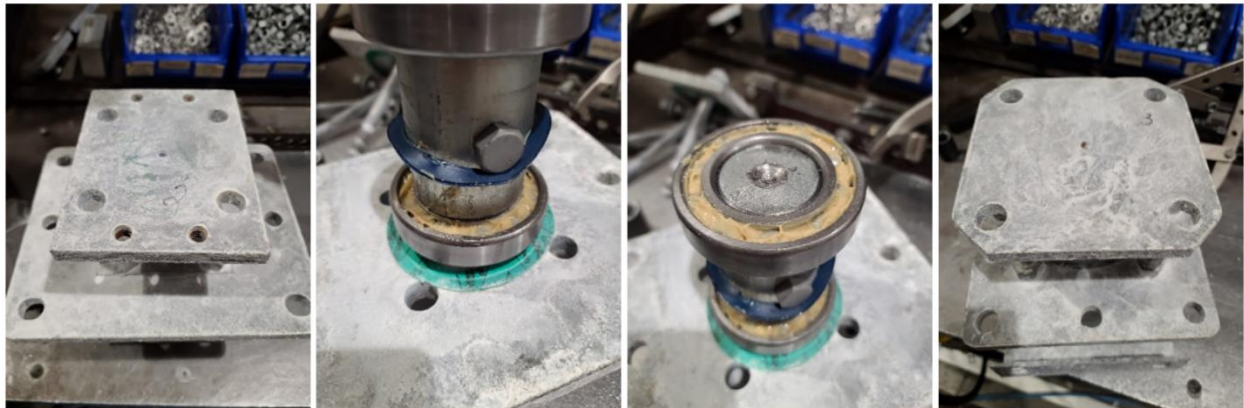
Figure 12: UUT2 Post-Tests 1–4 Interior and Bearing Condition
