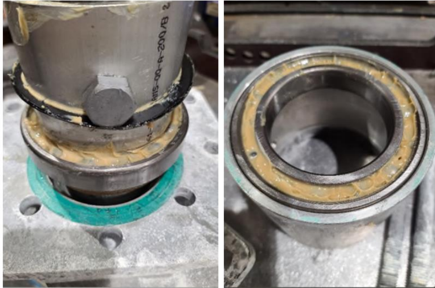
Figure 13: UUT3 Post-Tests 1–4 Interior and Bearing Condition
