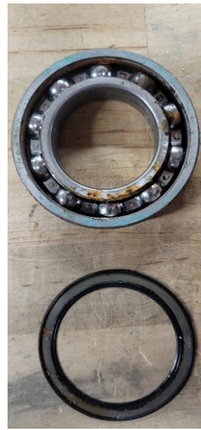
Figure 20: UUT6 Unvented Bearing, Forced Humidity Post-Test Condition
