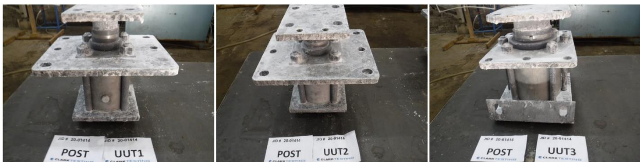
Figure 10: Salt Spray Post-Test Condition
