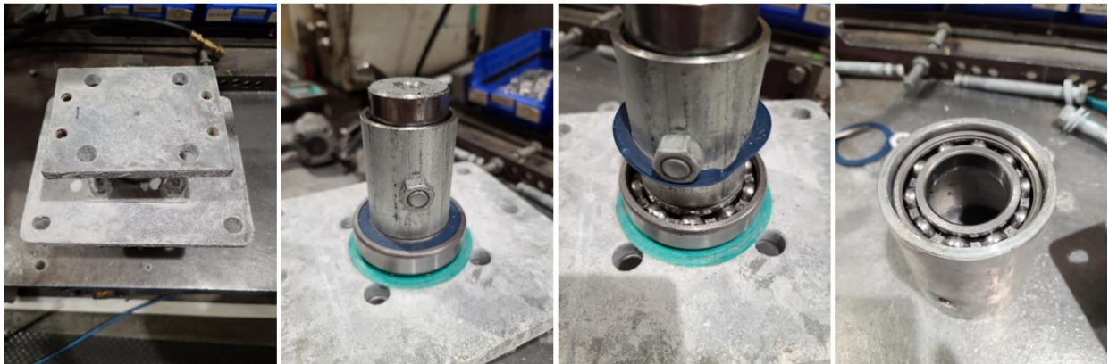
Figure 11: UUT1 Post-Tests 1–4 Interior and Bearing Condition
