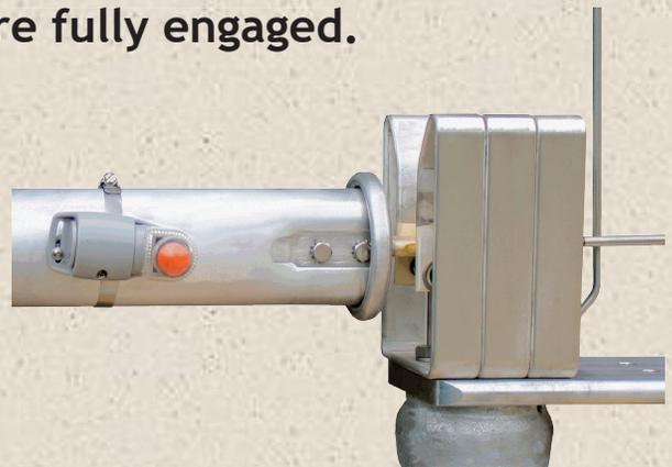
The colored ball indicates that the blade is closed to the full depth of the break jaw.
