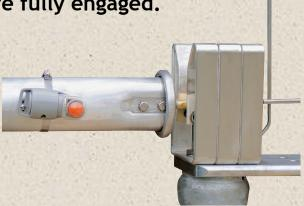
The colored ball indicates that the blade is closed to the full depth of the break jaw.
