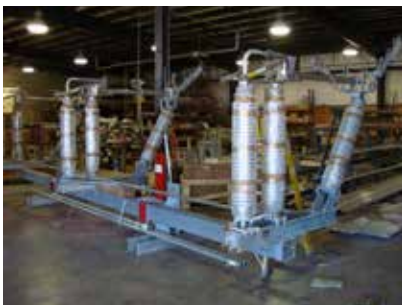
Unitized switch assembled at the factory.
