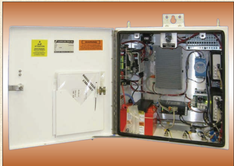
SPS containing (2) radios, a DigitaLogic IGIN, DigitaLogic IDAS, an I/O module, and optional radio kill switch
