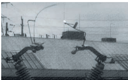
10 ms. The arc is completely extinguished.
