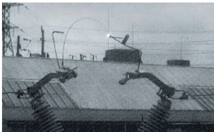
0 ms. Whip contacts are just beginning to separate. A slight spark can be seen.
