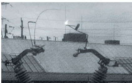
6 ms. The arc starts to extinguish.
